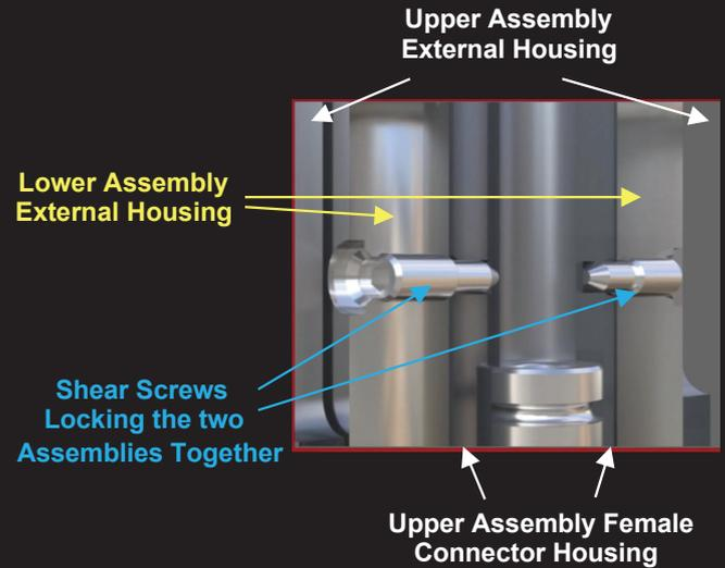
The PCLWF Adapter Tool Upper Assembly is slidden over the Lower Assembly until the Wet Connectors are fully mate before locking them together using two shear screws designed to break at a pre-determined tension. The wireline cablehead is then attached to the PCLWF Adapter Tool before running the toolstring in the hole.
